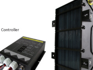
Semi-integrated 1kW fuel cell system Includes: • LCD display • Hydrogen sensor(optional) • Ambient temperature sensor • DC-DC converter • Ultra capacitor bank • Electronic control box • Electronic valves • RS232 connector • Blower controller • Start up battery connector • Software(optional) • ON/OFF switch • Emergency stop switch • PU tubing
